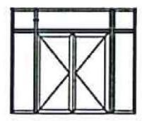
Doorsets incorporating side lights and/or fan lights may be constructed using a 'T-Bar' or 'Split Coupled Joint' method. Please see the data sheet for further details.
